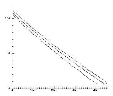
I have been able, for complicated reasons, to test three batteries sold as 9cell 90Whr batteries for the Dell Latitude E6410 computer, one made by Sanyo, one made by Simplo and one made by Samsung. The results of the test are shown on the graph.
