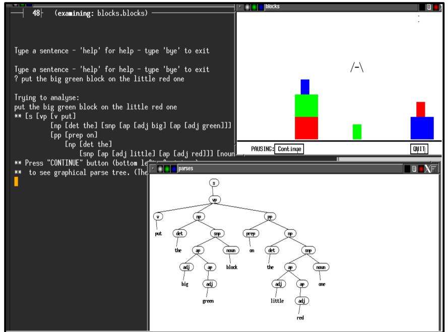
**Above:** how the machine understands a command "put the big green block on the little red one" -- showing the structure of the sentence diagrammatically. Having understood, it then makes a plan to achieve the goal. (The /-\ represents a hand!)
