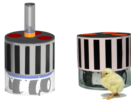
(a) The design of the PoulBot robot. The plexiglas bumper protects chicks fingers from been stuck in the robot's tracks
