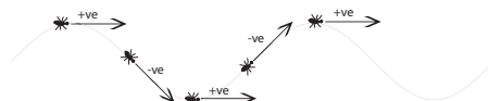
Figure 3. By weaving back and forth during locomotion it is possible to sample both the on-route and off-route views needed to train a classifier.
